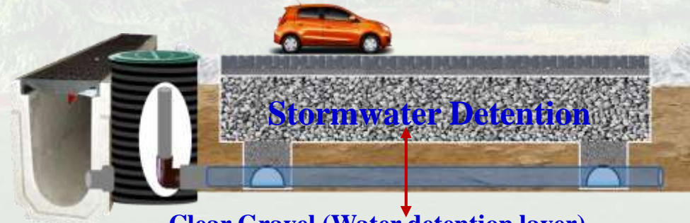
Clear Gravel (Water detention layer)
