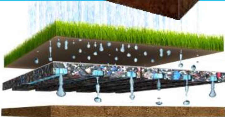
Sport field underground drainage
