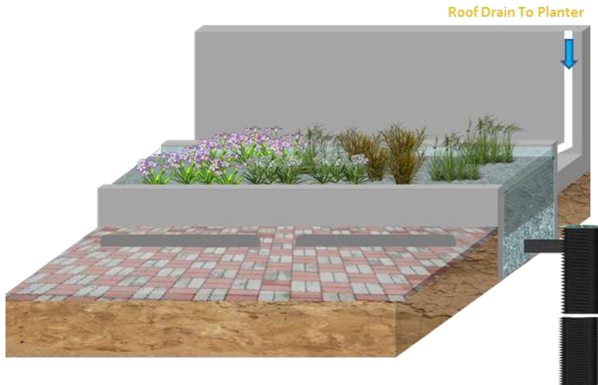
Stormwater Pretreatment Component—Roof Drain
