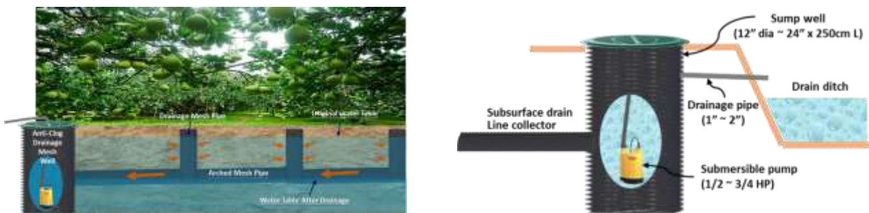
Figure 3. The soil water management for poorly drained agricultural land with artificial drainage.
