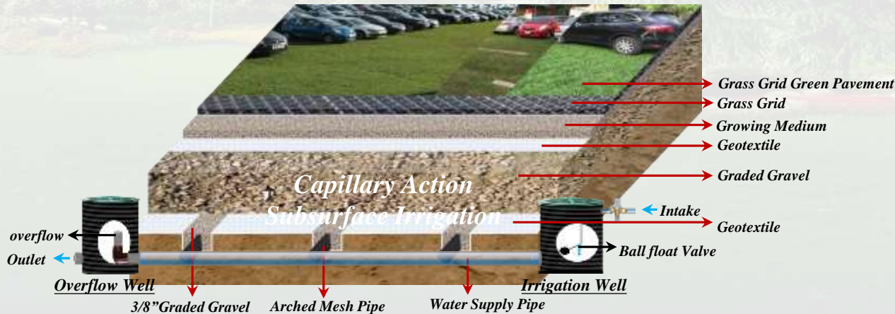
Grass Grid Green Permeable Pavement Parking Lot and Driveway Installation Steps
