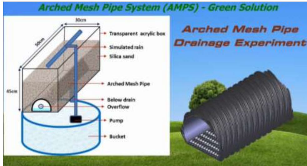
Arched Mesh Pipe Anti-Clog Drainage Demonstration
