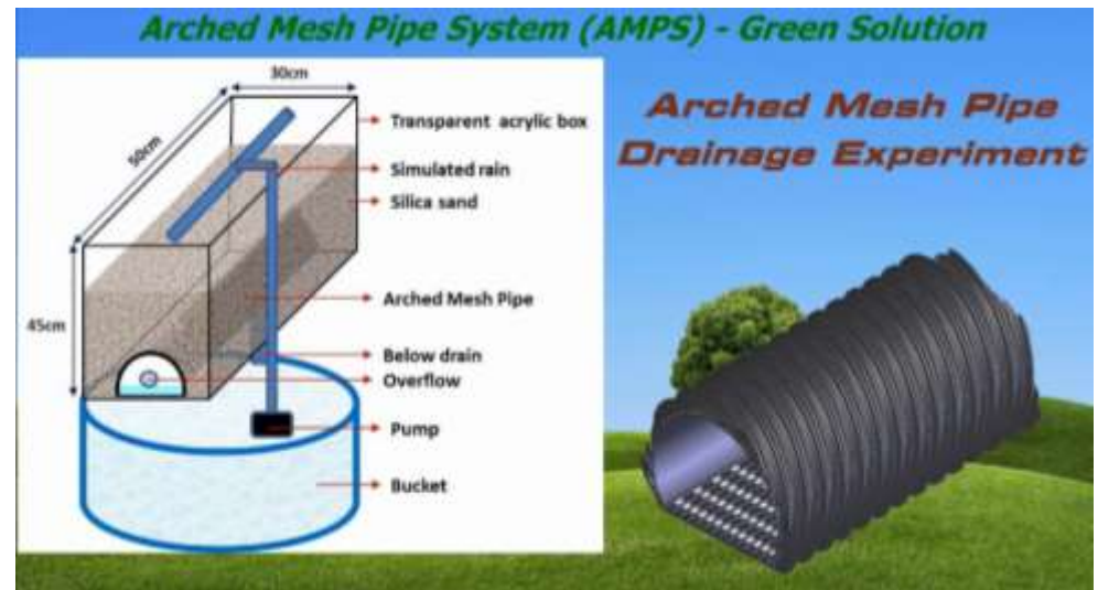
Arched Mesh Pipe Anti-Clog Drainage Demonstration
