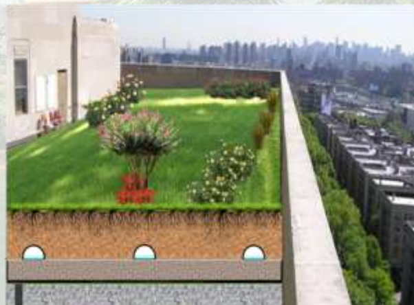
AMP-Arched Mesh Pipe-Green Roof Sub-Irrigated Raised System
