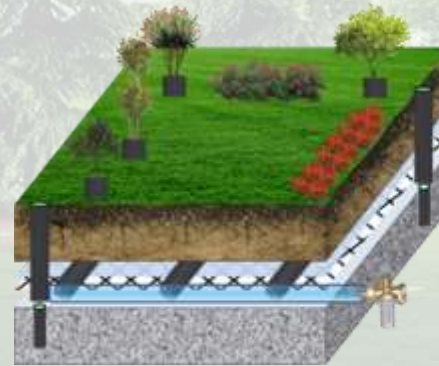
Green Roof AMP-Arched Mesh Pipe Sub-Irrigated Raised System
